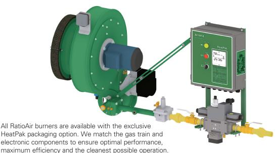
HeatPak packaging option. We match the gas train and electronic components to ensure optimal performance, maximum efficiency and the cleanest possible operation. Trilogy T420 Flame Safeguard controls with valve proof of closure and a metal NEMA 12 enclosure are included as standard equipment. The customer simply connects a regulated gas supply and electricity and the RatioAir is ready for operation.
