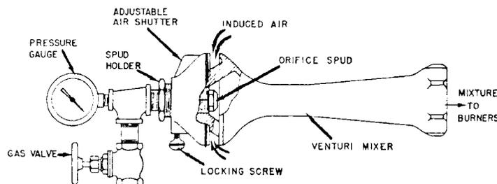
5. Complete the initial adjustment of the air shutter in the following manner.
