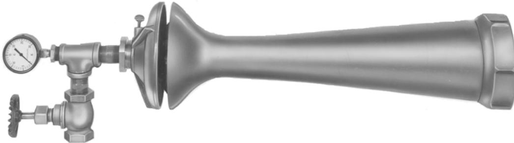
The Hauck AIG Series High Pressure Gas-Air Inspirators are ideal gas-air mixers designed for use with gas pressures ranging from 5 to 30 psig. The AIG inspirator uses the gas's potential energy, which is converted at the jet to kinetic energy, to entrain atmospheric air for combustion. After an initial adjustment of the air shutter the desired gas-air ratio is maintained.
