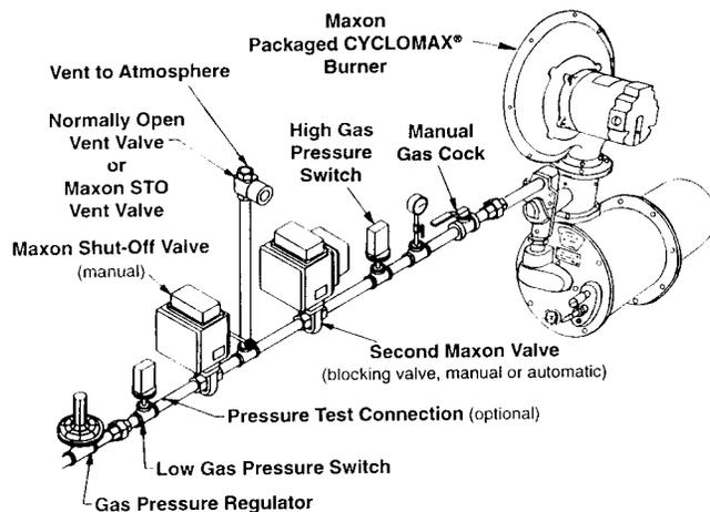
**Packaged CYCLOMAX® Burner** comes complete with its own combustion air blower. The burner also provides fuel flow control and a fuel/air mixing device.
