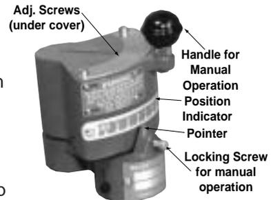
After the initial adjustment pass, adjust only the screw corresponding to the actual position of the MICRO-RATIO® Valve and the NEXT adjacent screw to be adjusted (either up or down the ramp). If possible, do not adjust the previous screw. Two passes through the firing range is enough. Some sensitive applications may require three passes with adjustments to get the ramp smooth enough to produce repeatable gas pressures at each setting.
