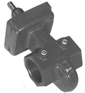
Normally-closed shut-off valves utilize power to open. Removal of electrical signal allows instantaneous release of the holding mechanism, allowing the powerful closing spring to close the valve in less than one second.
