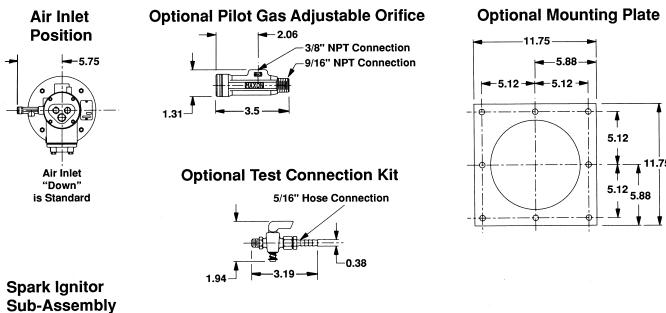
Pipe threads on this page conform to NPT (ANSI Standard B2.1)
