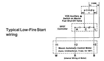
Regardless of the type of automatic control (highlow or modulating), Series "67" TUBE-O-FLAME<sup>®</sup> Burners should be at or very near the Low firing position for pilot ignition and main flame light-off.
