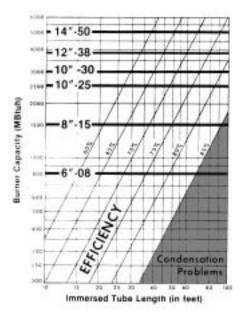
Many factors affect overall system efficiency. Tube length is the most important. The graph above shows approximate tube length required to attain a given efficiency. Typical installations run in the 70% – 75% range. Space considerations (including tube displacement) may limit possible tube lengths and so reduce efficiency. Above 85% efficiency, there is a risk of condensation-caused tube damage.
