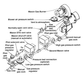
**TUBE-O-FLAME® Burner** provides the air supply (unless it is an LB version, which requires a separate combustion air blower). It also serves as a fuel flow control and fuel/air mixing device.
