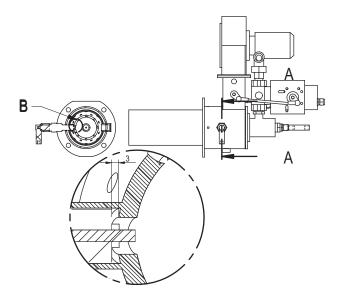
The spark ignitor can be mounted in 3 different positions on the burner housing: left, right and bottom (if the air inlet is on top). Spark ignitor replacement: insert the spark ignitor through the collar into the burner. Insert the spark ignitor in the cone bushing until its ceramic touches the cone - then retract the spark ignitor 3 mm to establish proper gap.
