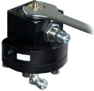
7) Remove the nut together with the disc and the diaphragm
