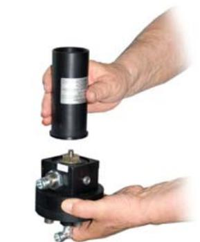
6) Unscrew the fixing nut
