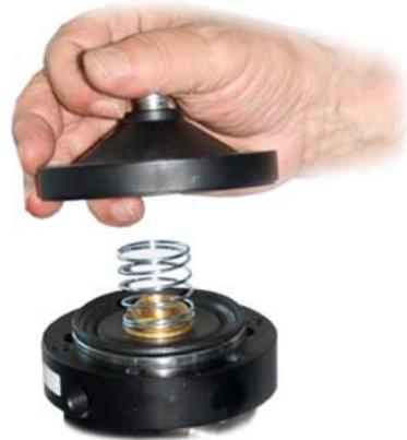
10) Remove the spring and the diaphragm
