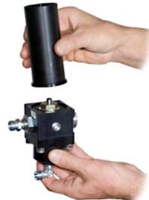
6) Unscrew the fixing nut
