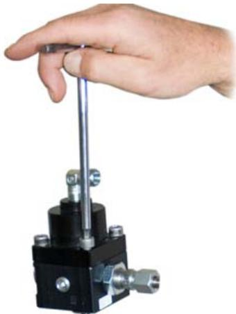
9) Remove the head cap together with the spring
