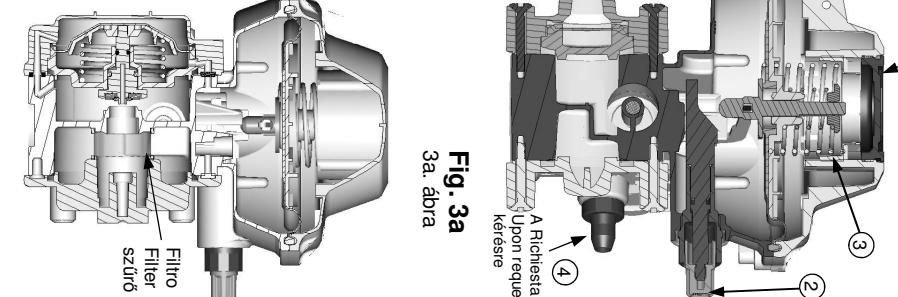
**Fig. 3** **CROSS-SECTIONAL DIAGRAM OF THE TWO-STAGE PRESSURE REGULATOR (FE)**
