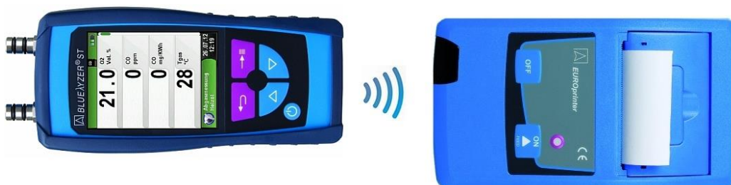
Fig. 3: Positioning of the BLUELYZER® ST towards the printer
