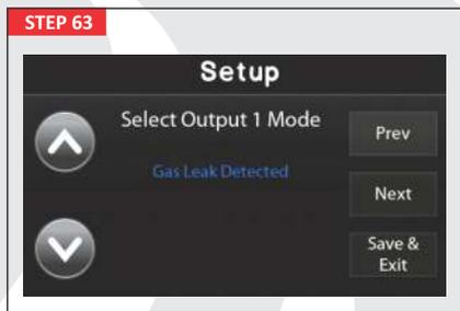
Gas Leak Detected - Output will be active if the Gas Detector goes into alarm indicating that there is a gas leak present within the room.
