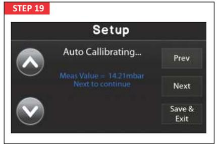
The unit will then close the gas valve and display the current gas pressure value.
