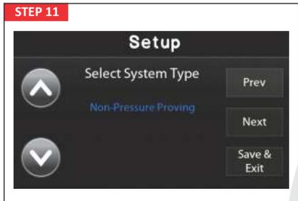
**Non-Pressure Proving** - is our non-pressure proving gas safety controller.
