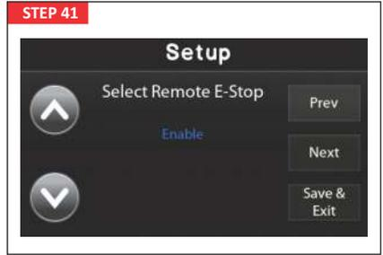
When enabled, the system looks for a dry (volt-free) contact from an Emergency Stop button. This contact can be wired in series with multiple E-Stop buttons.
