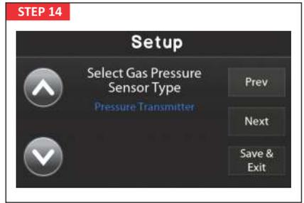
2. Gas Pressure Transmitter - Enables real-time pressure readings and improved leak and pressure detection ability.
