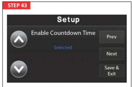
If enabled, the system will prompt for the desired run time (from 5 minutes to 8 hours) on each gas startup.
