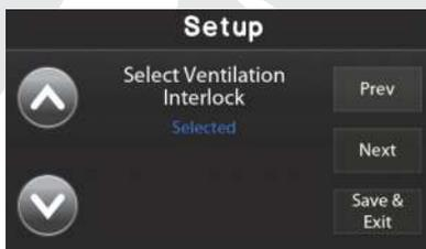
When the system is in the "Selected" state, it actively seeks a ventilation input and activates the fan contacts on the control board accordingly. Note: Fan output on the board is to drive your fan relay only, it does not provide power supply to the fan motor.
