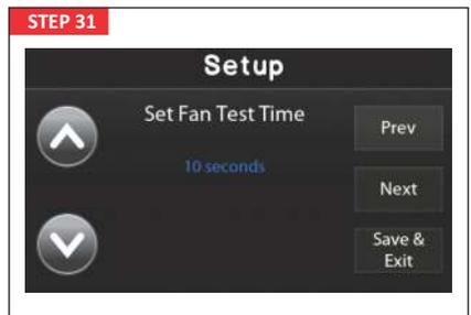
Fan test time is the time required for the fan to start and for the system to reach the minimum set air flow or pressure.
