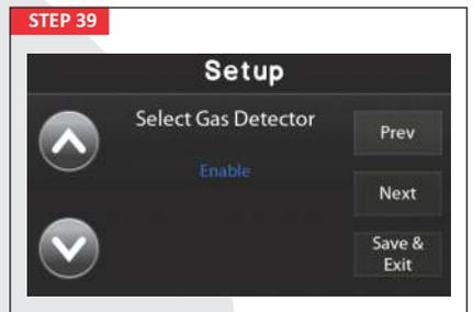
When enabled, the system looks for a dry (volt-free) contact from a gas detector.
