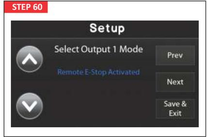
Remote E-Stop Activated - Output will be active only when a Remote Emergency Stop button has been activated.
