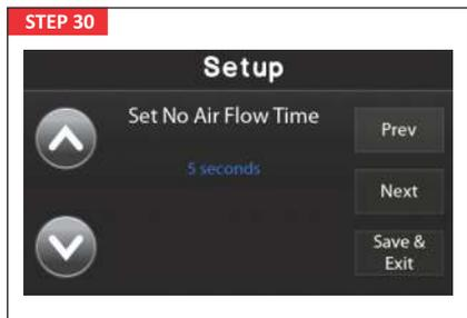
This is the time the unit will check the system to prove that the fan is not operating, is in a zero flow condition, and the Air Flow sensor is reading zero.
