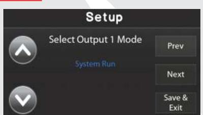
System Run - Output will be active when the system is on and running. This will become active after a successful test procedure.
