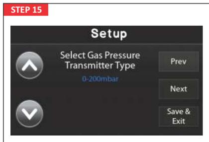
Gas Pressure transmitter is available in three ranges
