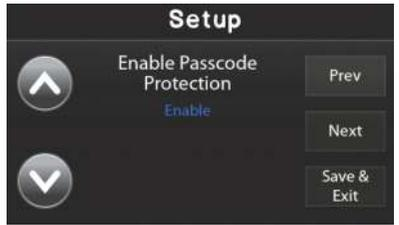
When enabled, a passcode is required each time gas is to be enabled. This can remove the need for physical keys to operate your system.
