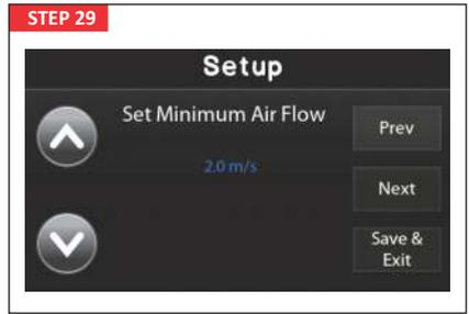
If Air Flow Transmitter is selected, the system will ask you to set the minimum airflow the unit requires before a fault will occur.
