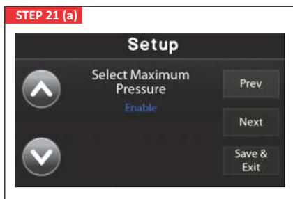
When enabled the system is looking for a maximum gas pressure.
