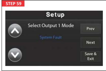
System Fault - Output will be active when the system is in fault. This will become active after a fault or warning in the system.
