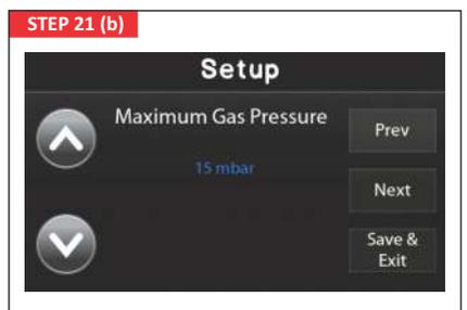
Set the maximum gas pressure here. Above this value, the system will automatically trigger a High Gas Pressure fault. Note: This option is only available if a pressure transmitter is installed.
