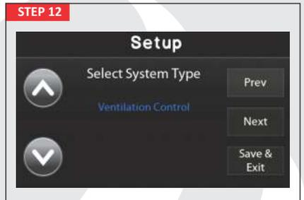
**Ventilation Control** - as a ventilation control box to ensure gas can only be supplied when ventilation fan is running. This is a non-pressure proving system.
