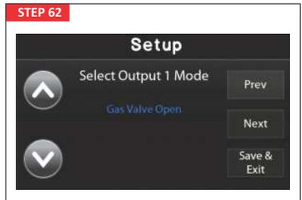
Gas Valve Open - Output will activate when the gas valve is open. This includes during the testing period when the gas valve pulses to allow pressure testing.
