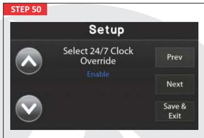
When enabled, the 24/7 clock can be overridden to accommodate gas usage requirements outside normal hours, requiring a unique password to be set.
