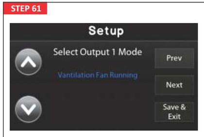
Ventilation Fan Running - Output will be active when the Ventilation fan is running, this includes during the testing period when the fan flow is being proved.
