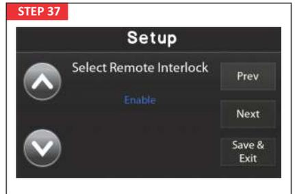
When enabled, the system will search for a remote 24-240VAC, or 24VDC input.
