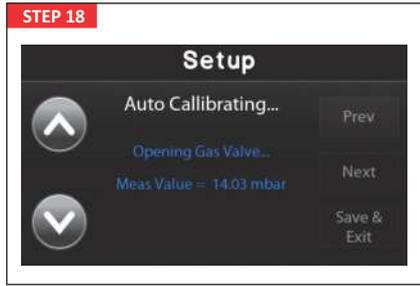
The unit will then open the gas valve and pressurise the system. **SAFETY NOTE:** Gas will now be in your downstream pipework.
