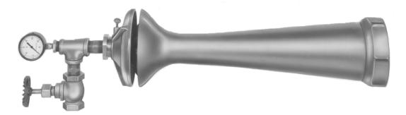
The Hauck AIG Series High Pressure Gas-Air Inspirators are ideal gas-air mixers designed for use with gas pressures ranging from 5 to 30 psig. The AIG inspirator uses the gas's potential energy, which is converted at the jet to kinetic energy, to entrain atmospheric air for combustion. After an initial adjustment of the air shutter the desired gas-air ratio is maintained.
