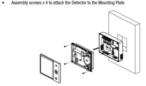
The Mounting Plate contains the terminals for connecting the power supply and relay outputs. Once the connections are made, the detector simply plugs into the Mounting Plate.
