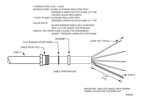
Fig. 3. C328 cable preparation.
