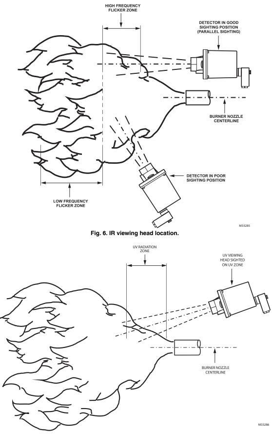
Fig. 7. UV viewing head location.
