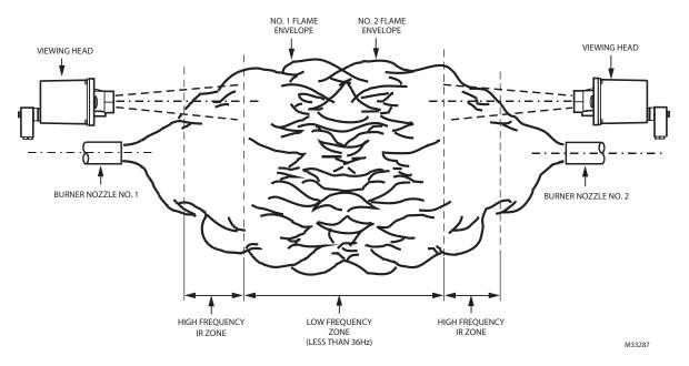
Fig. 8. Sighting opposed fired burners.
