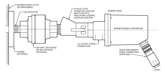
Fig. 10. Viewing head mounting example 2.
