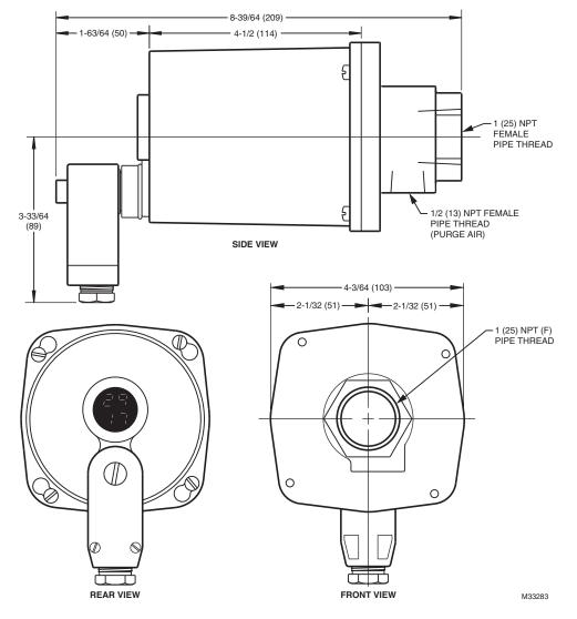
Fig. 4. S550B, S552B and S556B dimensions in in. (mm).
