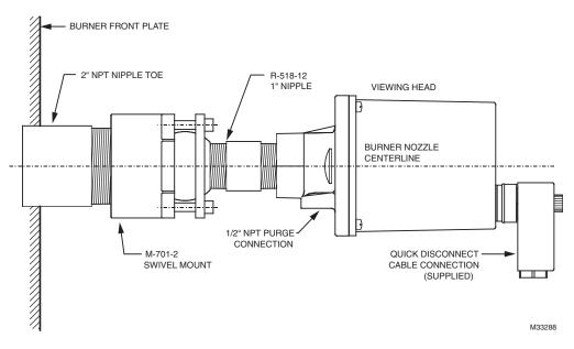
Fig. 9. Viewing head mounting example.
