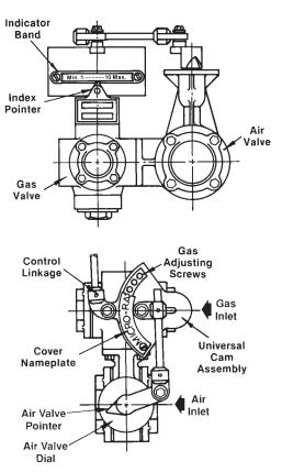
Having marked and/or recorded the MICRO-RATIO® Control Valve's air valve settings for both minimum and maximum firing positions, you may adjust the linkage and travel of the gas valve's stroke (see sketch below).
