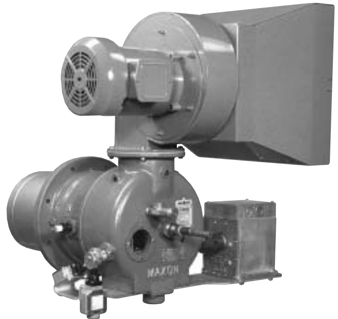
Model 415 OVENPAK®-II Gas Burner with optional combustion air filter, high and low fire position switch set, spark ignitor, provision for customer's UV scanner and with connecting base and linkage for electrical control motor
