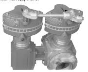
Rotate the air valve while watching the manometer for the minimum air differential pressure of 0.1" wc. (Note: This is a very small increment on a normal manometer. Readings/ settings above 0.1" wc will lessen turndown ratio of burner system.) Then mark red air valve dial (see sketch below) opposite crank pointer.
