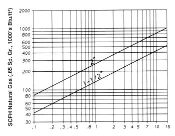
Differential Gas Pressures (measured between gas test ports G<sub>1</sub> and G<sub>2</sub>) in inches w.c.
