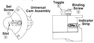
Loosen Allen set screw [1] and binding screw [2] in toggle [4]. Move the toggle in universal cam assembly slot towards the center of rotation so that gas valve can rotate from its minimum to maximum position, while the air valve swings between the established (and marked) minimum and maximum settings.
