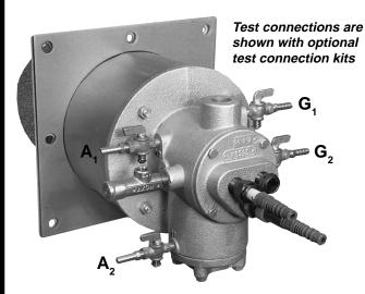
**Combustion air differential pressures** read across burner's built-in air test connections  $A_1$  and  $A_2$  (shown in photo above) are shown in Chart 2. Note that graph for 2" RAMFIRE® begins at 0.2" wc differential. This is required minimum for 2" size.
