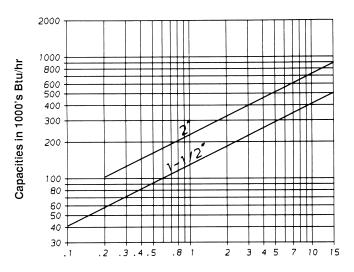
Differential Air Pressures (measured between air test ports A, and A,) in inches w.c.
