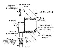
Burner block and casting failure is frequently the result of external stresses and strains transmitted to the burner through the piping. Flexible connections are recommended in all piping to reduce piping stresses and alignment/shifting problems. Installation of such connectors at certain key spots in the air or gas manifolding can prevent damage to the burners from uneven thermal expansion.
