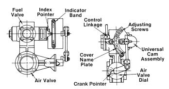
8. Establish the maximum combustion air differential pressure by moving MICRO-RATIO® Valve assembly toward the higher numbered positions until the desired air differential (in accordance with burner specifications) is reached. Again, mark red air valve dial opposite crank pointer (refer to Chart 2 on page 4300-S-9).
