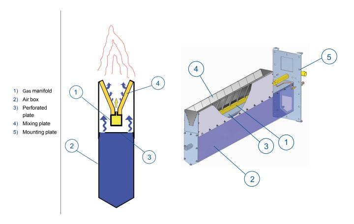
An additional perforated plate ensures the combustion air is distributed evenly over the entire burner length. This results in a stable and even flame pattern.
