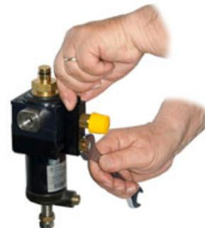
6) Remove the DAMPER device
