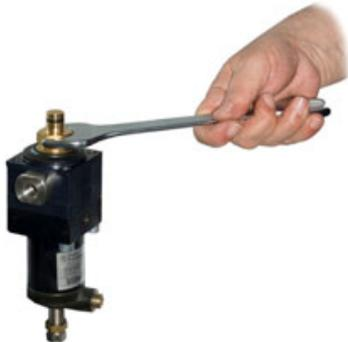
8) Remove the support and the diaphragm
