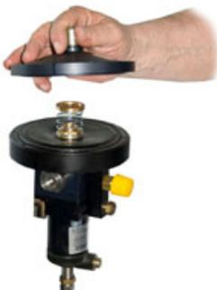
3) Loosen and remove the fixing bolts of the flange to the body
