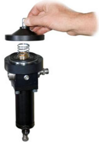
10) Remove the spring and the diaphragm
