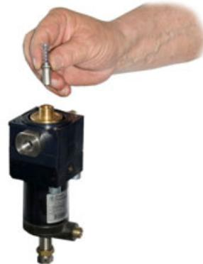
10) Loosen the blocking nut and totally unscrew the pilot regulation bolt
