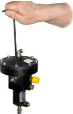
2) Remove the high cap together with the o'ring, the spring and the diaphragm with appropriate disc
