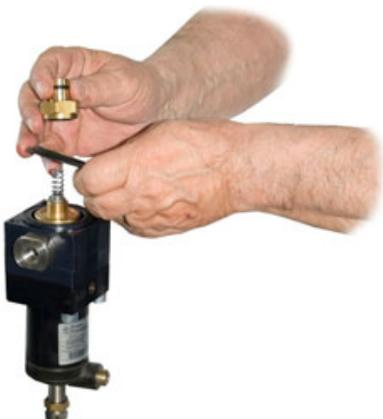
9) Remove the diaphragm and the spring
