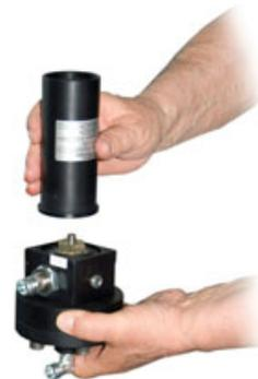
6) Unscrew the fixing nut
