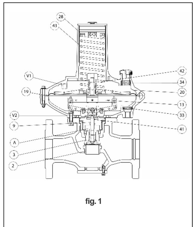
In fact, this solution allows the diaphragm protection disc 20 to rest on the upper stroke end V1 exceeding the load of the spring 42 and thus releasing the obturator from the load resulting from the sudden pressure increase.
