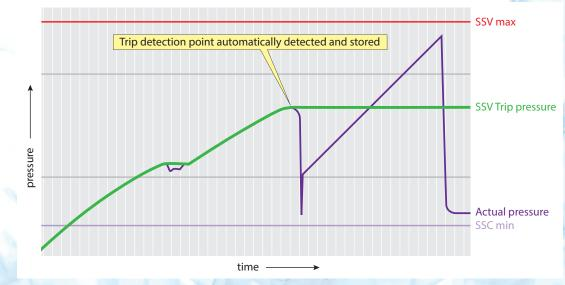
Magnetic sensor Automated trip detection
